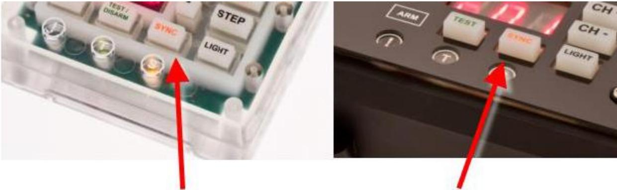
**Hold down SYNC buttons for 3 seconds together until the LED blinks quickly**
