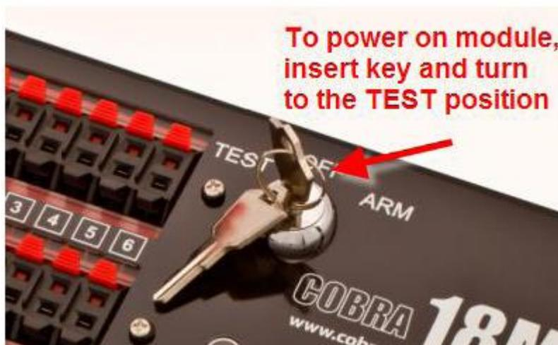
When the firing module is powered on, the following information is displayed:
