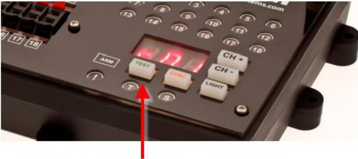
**Press and hold to test continuity and display module address**
